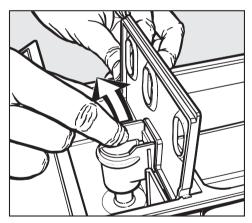
Remove the siphon tube from compartment <u>18</u>.
